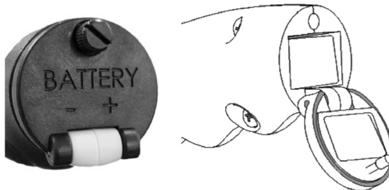
Figure 8. View of Battery Door and Compartment
