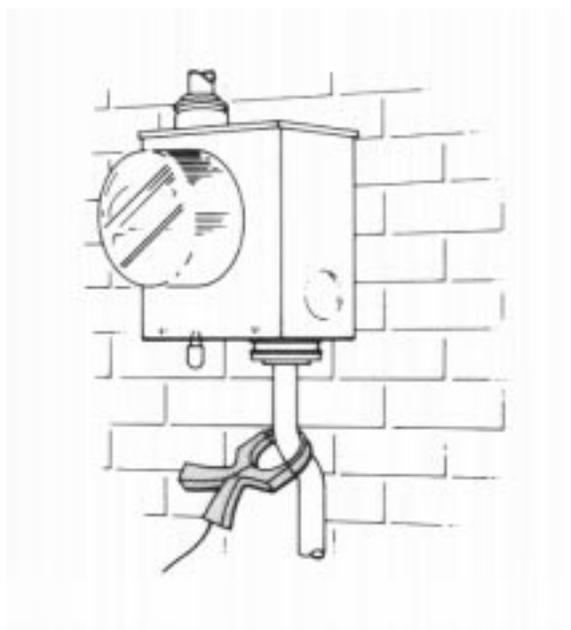
Figure 4-6. Inductive Signal Clamp Hookup
