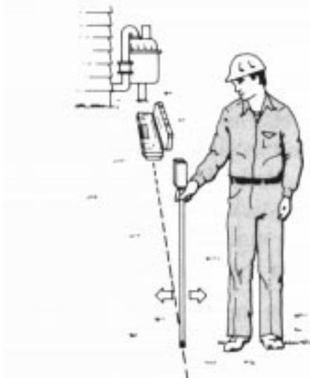
Figure 4-9. Inductively Coupled Tracing Signals
