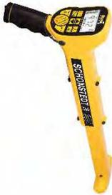
In sonde mode, the transmitter is not used at all. This mode is used to trace non-metallic pipes, or metallic pipes where other modes are inapplicable or inefficient. A small beacon transmitter, or sonde, is pushed through the pipe, and the receiver searches for the signal emitted by the sonde.
