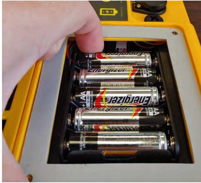
Once the battery pack has been removed, replace all 10 AA batteries with a new, matching set. Do not mix new and old batteries or batteries from different manufacturers. After replacing the AA batteries in the battery pack, place the battery back into the compartment, allowing the wire to stick out of the compartment, then tuck the excess wire into the cavity around the connector. Finally, replace the cover and the screws.
