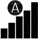
If the "A" is not visible, the receiver is operating in the manual gain mode; therefore, a means to show the user the relative gain setting is necessary. The bar graph indicates the relative strength of the gain.
